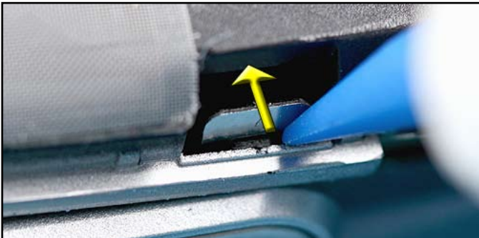
17. Place the SS-93 between the B-COVER edge and the clip of the FLIP MODULE and release it carefully.
