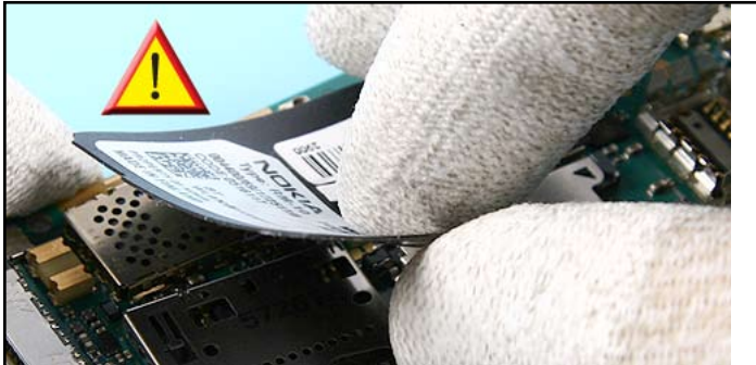
46. Remove the BATTERY DECK. Do not use too much force.
